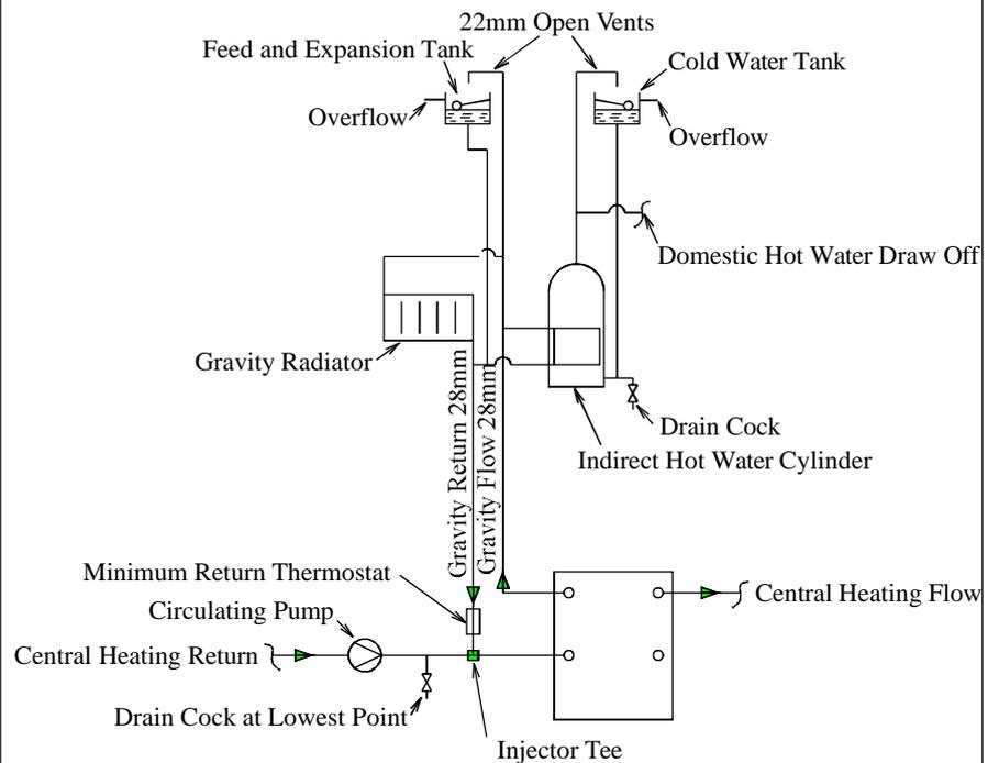
Fig. 6. Typical Central Heating & Hot Water System
