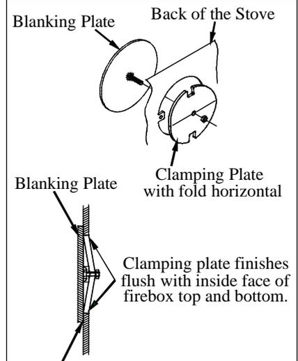
Fig. 12. Flue Blanking Plate.
