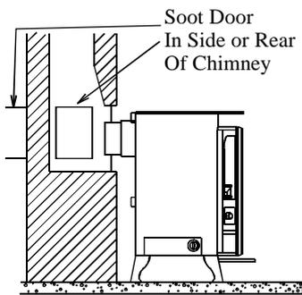
Fig 8. Vertical Register Plate With Bricked Up Fireplace
