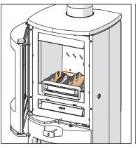
Once kindling is alight, add smaller logs. Keep air control fully out and close door
