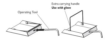
For optimum wood burning, it is important to leave a layer of ash around 1cm thick on the base of the stove. Before removing ash ensure that it has cooled down,
