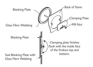
webbing fitted to its sealing face, and fitted to the rear flue outlet. Ensure that the fold on the clamping plate is in line with the lugs on the firebox as shown in Fig 11. Ensure that the clamping plate does not prevent the throat plate from seating correctly. All flue connections must be well sealed. The top outlet connection is made directly to the cast top of the Arc 7 model, the Arc 7 is supplied with a flue collar for rear outlet installations.
