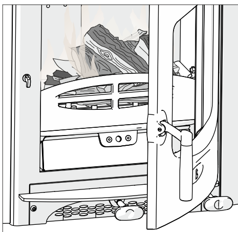
Fig. 5 Building up the fire
