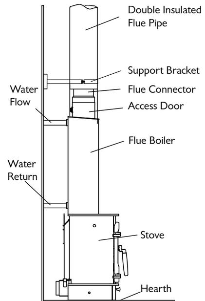
Fig 7. Horizontal Register Plate Into Conventional Chimney
