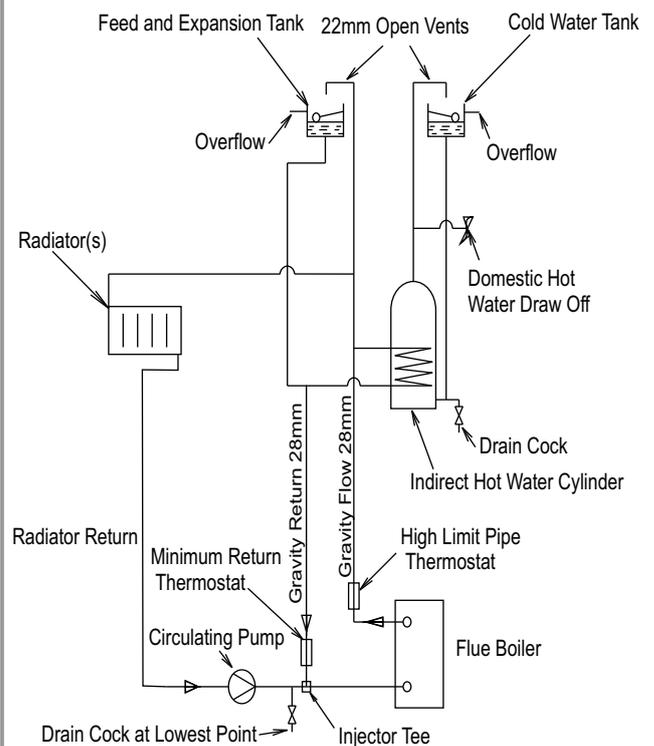
**Fig 3. Larger System With Heat Leak Radiator Controlled By High Limit Pipe Thermostat**
