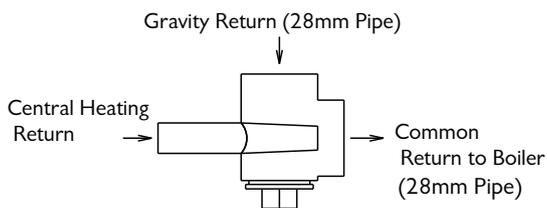
gravity flow pipe, which gives priority to the domestic hot water, but brings the pump on to heat the radiators when the flow pipe temperature exceeds the set temperature. A minimum return pipe thermostat will prevent cold water being pumped around the circuit
