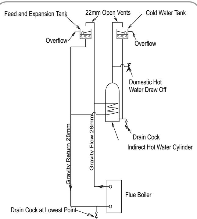
**Fig 2. Basic System Where Heat Leak Radiator Is Not Required**
