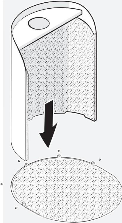
Secure with the five hex head screws through the slots in the back into the attachment lugs on the base using the allen key.
