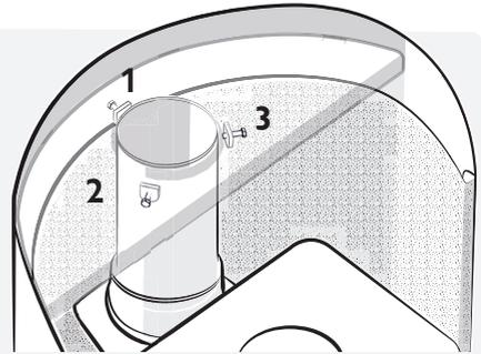
If required for installation, the stove pod shelf can bear a static load of up to 56kg
