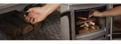
Fully open the air control for maximum air intake and a quick and easy ignition. Light the fire lighter.
