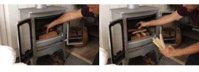
Place 2-3 smaller logs on the stove bed. On top of this build a *Jenga* stack of 6-8 kindling sticks and place a natural fire lighter inside.
